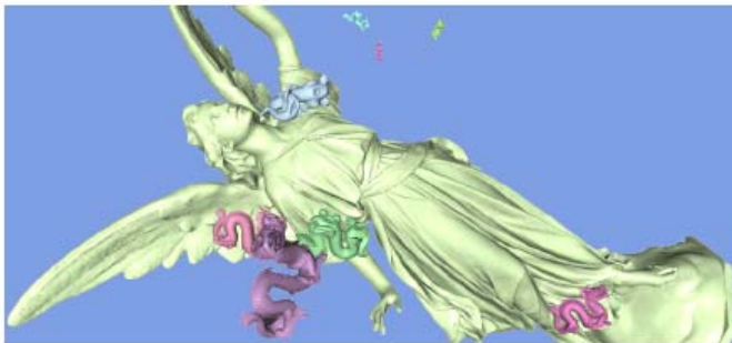
Figure 9: Dynamic Simulation: Dragons consisting of 800K triangles are dropping on the Lucy model consisting of 28M triangles. We obtain 2 times improvement by using COL on average.
